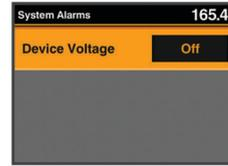
**Device Voltage:** Sets an alarm to sound when the battery reaches a specified low voltage.
