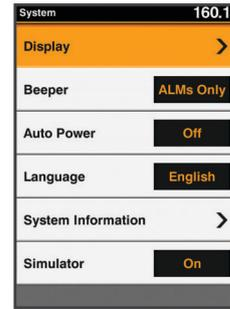
**Display:** Adjusts the backlight brightness (*Adjusting the Backlight, page 1*) and color scheme (*Changing the Color Mode, page 1*).
